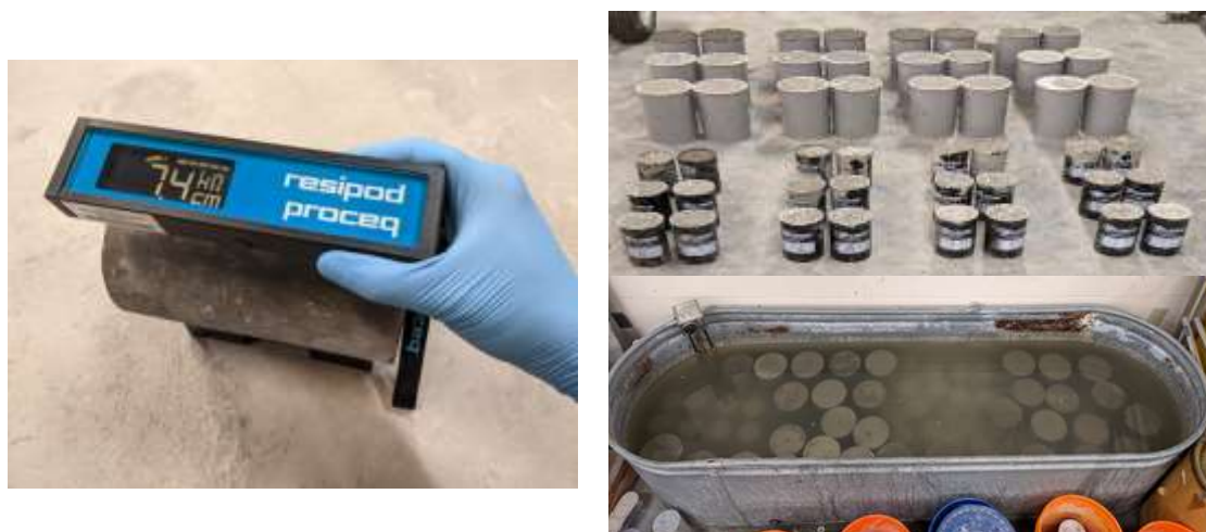
Figure 1. Surface Electrical Resistivity Measurement
