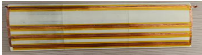
Figure 8. Plasma actuators positioned at the most optimum points
